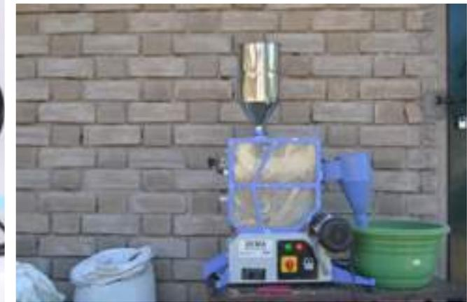
Efficient huller, polisher, de-stoner etc for remote tribal and rural areas- dependent on diesel (4 more machines ready to scale by quarter 3 2018-2019 - (co-developed by 3 different local entrepreneurs/ manufacturers)
