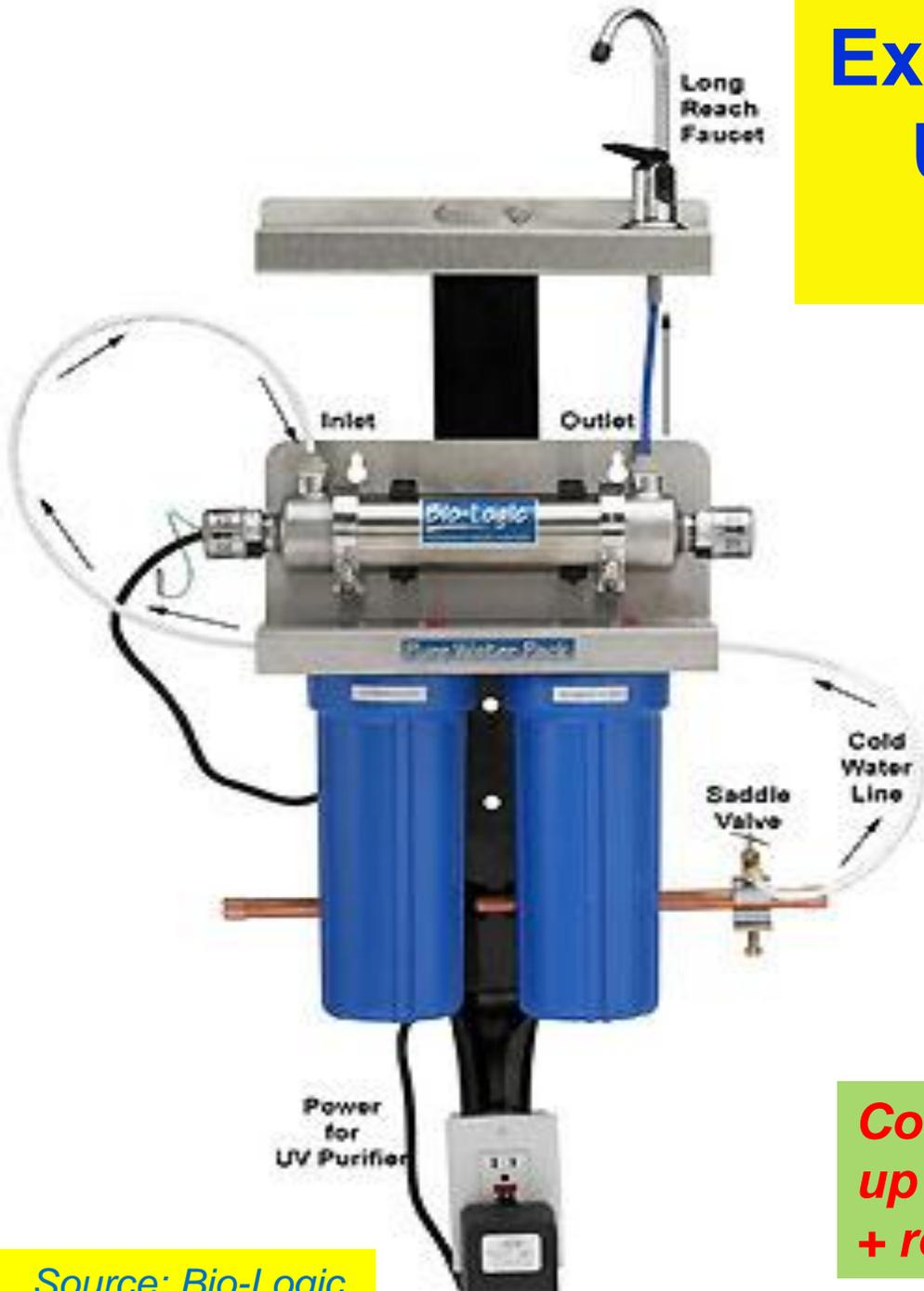
UV water purifier utilizes a germicidal short wave radiation lethal to microorganisms.
