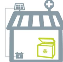
The super-efficient refrigerator requires just **10% of the solar panel and battery capacity** as the conventional solar vaccine refrigerator
