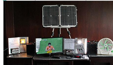
\*Systems provide energy for 4 lights, a 19" color TV, a radio, and mobile phone charging
